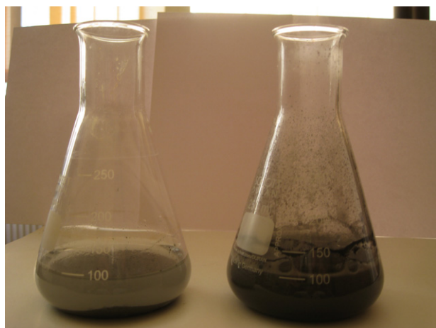
Fig. 4. Regular (left) and activated (right) aluminum dross powders in tap water at room temperature, the regular aluminum dross powder shows no apparent reaction, whereas the activated aluminum exhibits effervescent reaction with hydrogen release.
